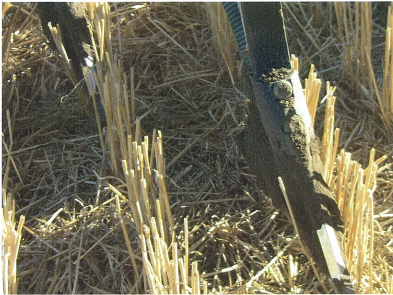
Figure 4. The “Stealth Paired row hoe” type seeding row opener mounted on the plot seeder shown on the stubble row, i.e., in the “On-Row” seeding orientation.
