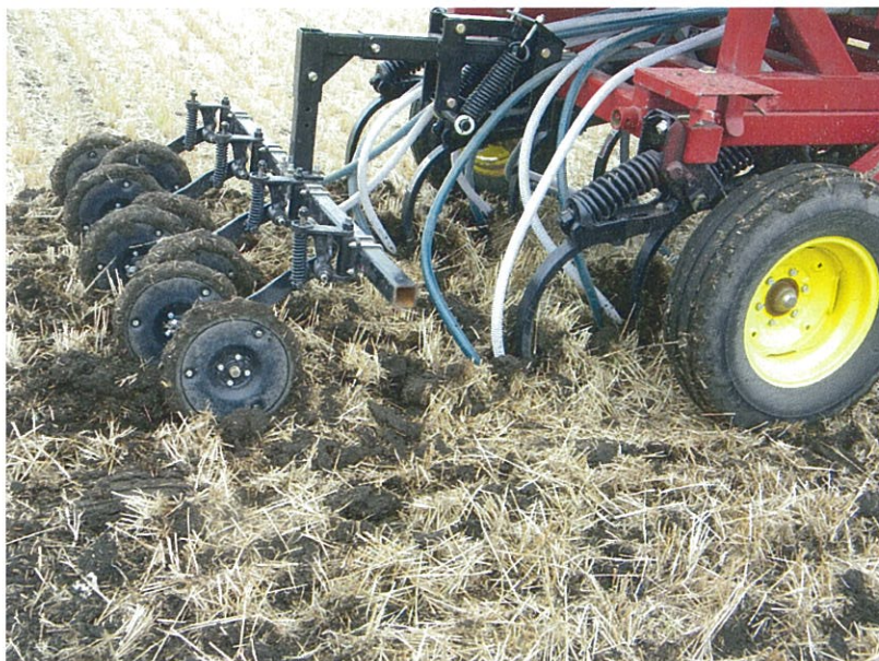
Figure 2. A general view of the “Stealth Paired row hoe” type seeding row openers mounted on the plot seeder.
