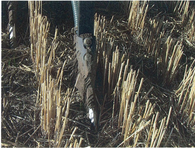
Figure 3. The “Stealth Paired row hoe” type seeding row opener mounted on the plot seeder shown between stubble rows, i.e., in the “Inter-Row” seeding orientation.
