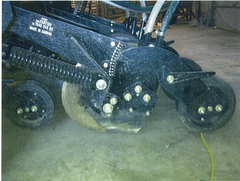
Figure 1. A general view of the “Pillar Lasers - disc hoe” type seeding row openers mounted on the plot seeder.
