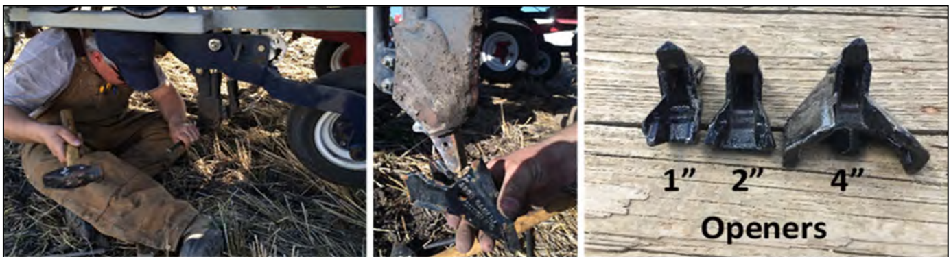
Fig. 2. Dutch Universal openers used in the study and how they are changed.
