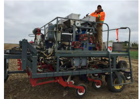
Fig. 1. Custom-made plot drill used to apply all treatments and seeding at all locations.
