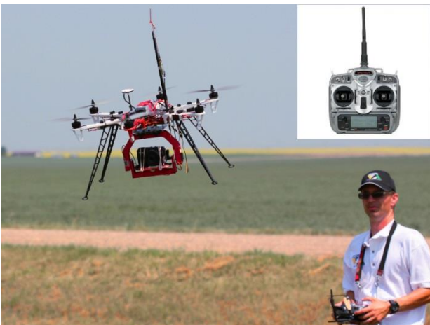
Figure 3. UAV operated via manual controls using a 2.4 GHz Spectrum DX7 controller.
