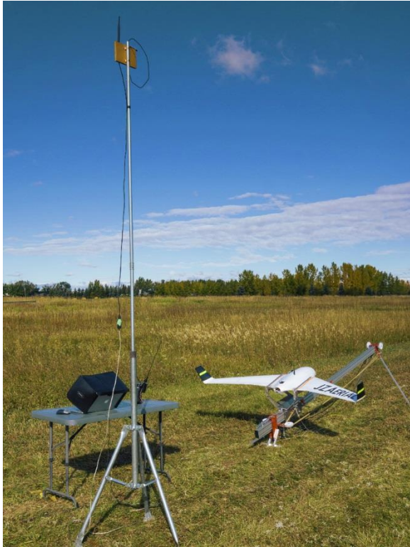
Figure 2. A ground telemetry module (GTM) connected to a laptop with a screen shade. The laptop runs the flight planning software and displays the position, altitude, speed, battery status and other information relevant to the operation of the UAV.
