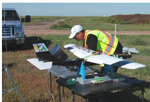
Figure 4. The custom build fixed wing UAV that was used for this project. It is equipped with a MicroPilot MP2028 flight controller, has 183 cm wingspan and weighs 2800g with camera payload.
