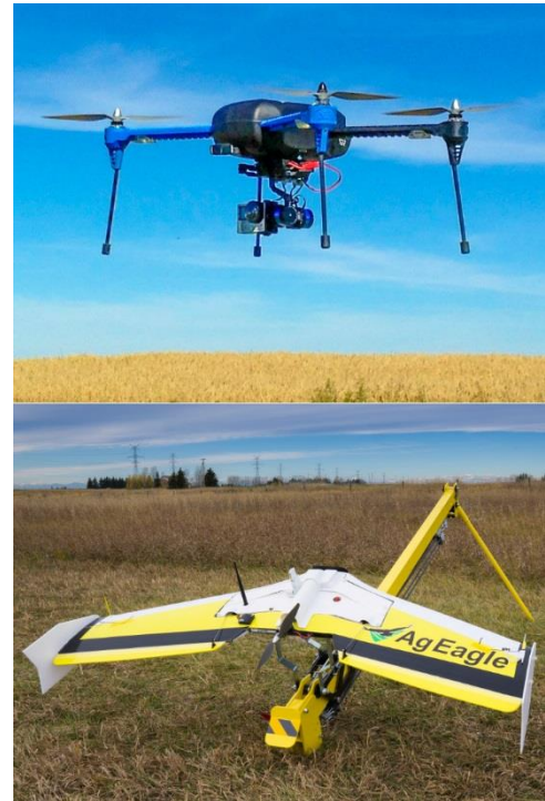
Figure 1. Multirotor and fixed wing UAVs of the type commonly used in agriculture.
