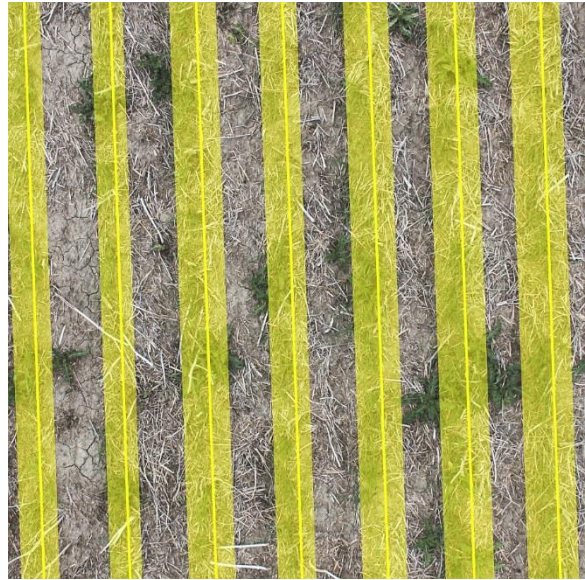
Figure 8. Delimitation of crop rows with the Hough algorithm.
