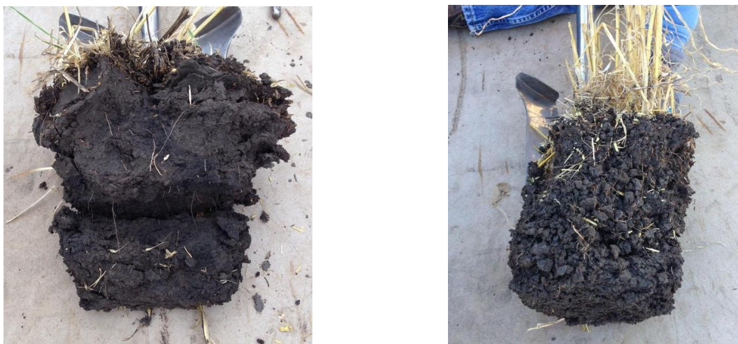
Figure 4. Morrin site: Soil structure under castor wheel left side and no traffic right side (photo Steve Larocque)
