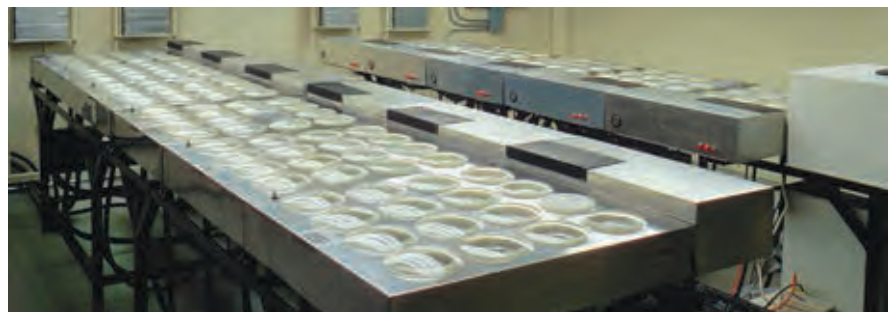
This thermal gradient plate is like 176 mini growth chambers. Researchers use it to quantify the process of seed germination, plant shoot emergence, insect growth and development, and plant and insect pathogen infections. From these data, they can quantify the ecological, biological, and climatological relationships that influence pest status.
