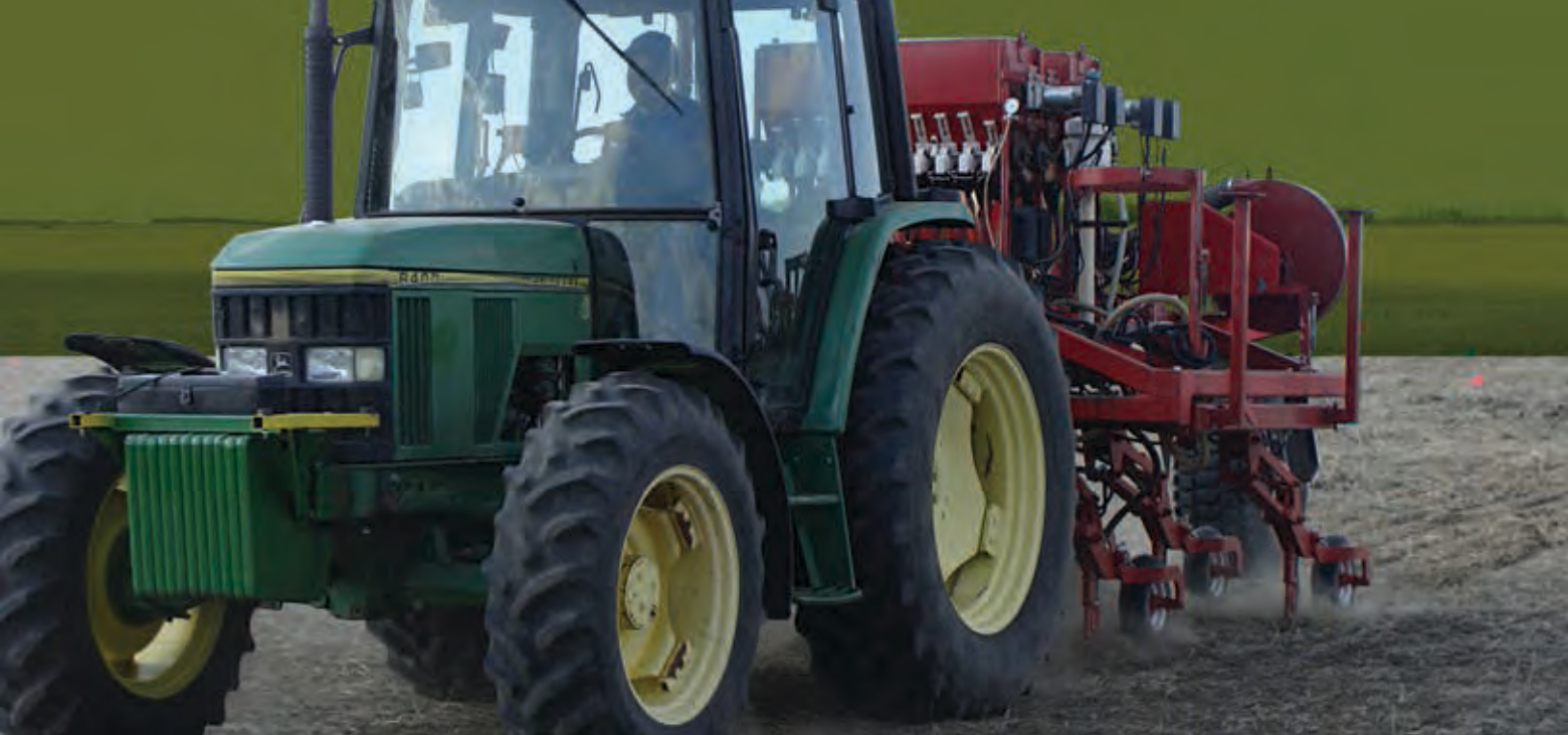
The small-plot study used a drill unit capable of attaching all six opener types, which avoided possible confounding effects such as drill weight, row spacing, seed metering system and packing system.
