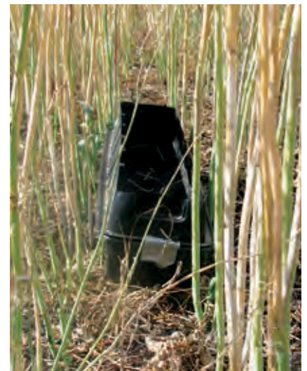
Trays used to determine pod-drop and seed-shatter in canola before harvest. In 2012, catch trays were modified by adding a top section to reduce possible predation and/or the effect of adverse weather conditions.
