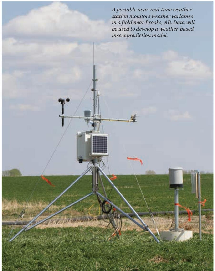
*A portable near-real-time weather station monitors weather variables in a field near Brooks, AB. Data will be used to develop a weather-based insect prediction model.*
