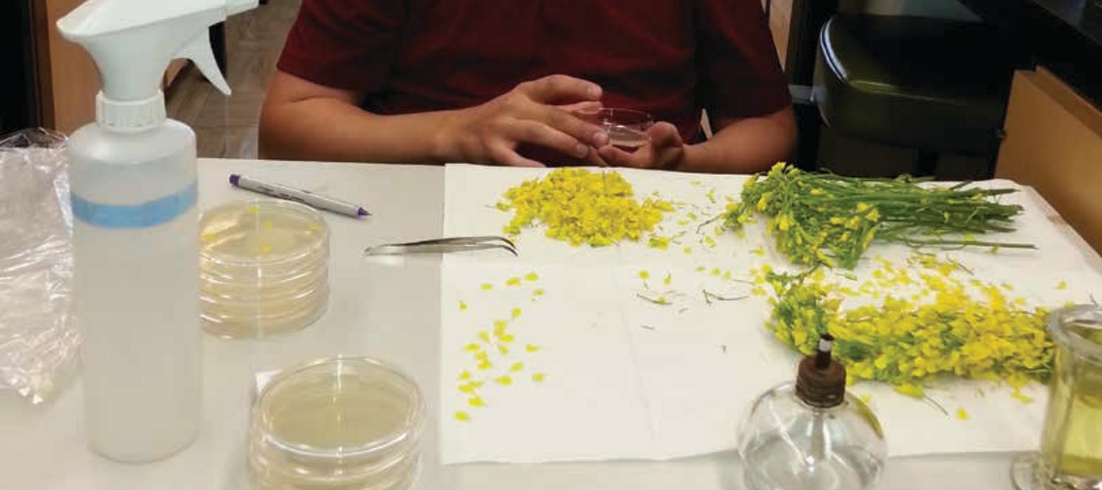
Researchers have developed a PCR-based method to measure the amount of DNA of the sclerotinia stem rot pathogen in canola petals.
